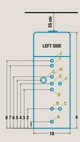
All connections are 3/4''(N) – Internal thread (Z) – External thread
